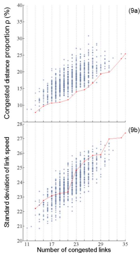
Fig. 9. The relationship between the congested distance proportion (a), the standard deviation of link speed (b) and the number of congested links.
