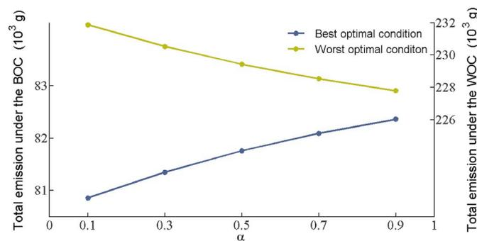
Fig. 5. Variations of the total emission at different  $\alpha$ -cut levels.
