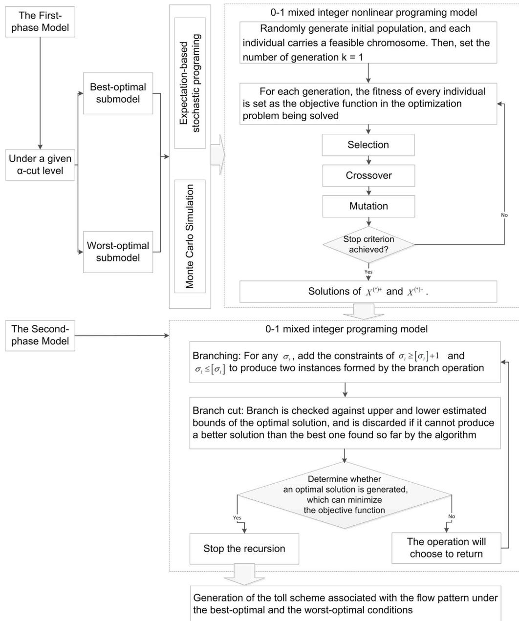
Fig. 3. The solution procedure of the TMPEP model under uncertainty.
