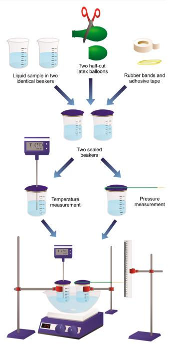
Vapor Pressure Measurement System
