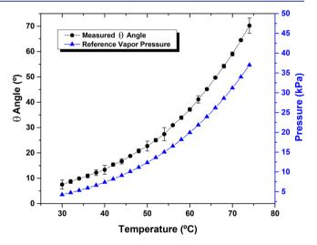
**Figure 3.** Double-*y* multicurve. The left-hand *y*-axis showing the angle as measured by the system, expressed in degrees, for deionized water as a function of temperature ( ${}^{\circ}$ C), which is shown on the *x*-axis. Vertical error bars refer to  $\pm 1$  standard deviation (n = 3). The right-hand *y*-axis shows the reference values for the vapor pressure of water (kPa) as obtained from the data tabulated in the *CRC Handbook of Chemistry and Physics*. <sup>55</sup>
