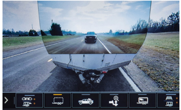
The Transparent Trailer View feature available on the 2020 GMC Sierra HD lets you “see” right through a towed trailer.
