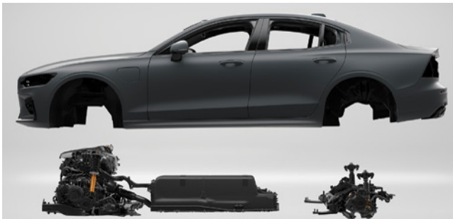
The Polestar Engineered variant of the S60 T8 shows the placement of the battery pack in the center tunnel.
