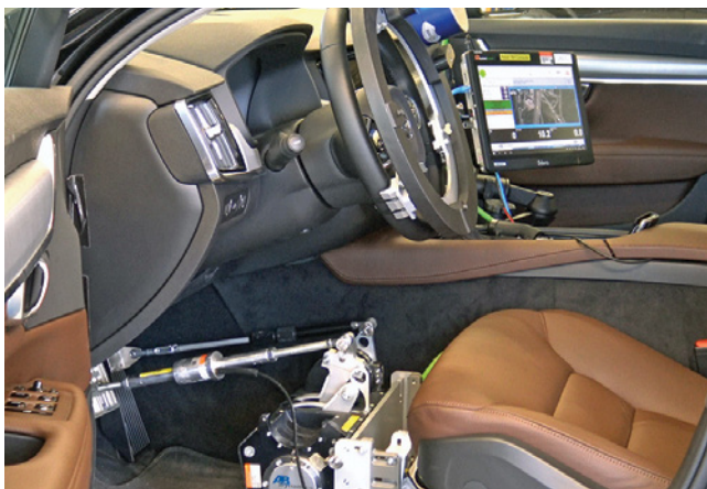
Typical robotic-driving hardware configuration. AB Dynamics' new Flex-0 does not replace it for all scenarios, can be a complementary system.
