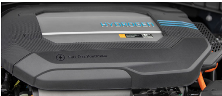
The fuel-cell stack on the 2019 Hyundai Nexo features an integrated air-processing system that helps make the FCEV as quiet as a typical BEV.
