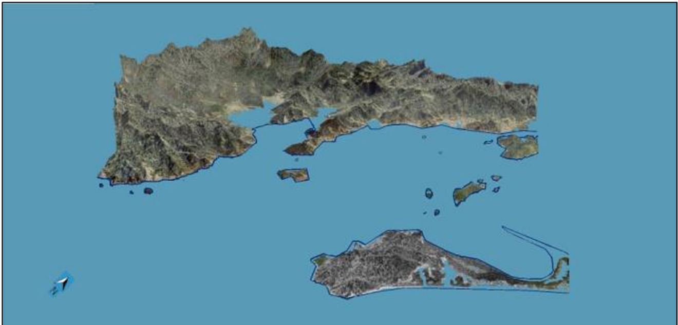
Fig. 4 Simulation of elevation of 2.15 m of sea-level visualized in the DEM elaborated for the study area (the current coastline is highlighted)
