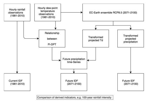
**Figure 1.** Approach for intensity-duration-frequency (IDF) construction including temperature scaling to derive future short-term precipitation extremes.
