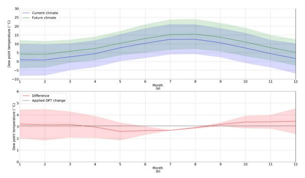
**Figure 3.** (a) Current and future monthly mean dew-point temperatures with 95% confidence intervals, and (b) monthly averaged increase in dew-point temperature under RCP8.5 with 95% confidence intervals. The black dotted line shows the increase in Td as used.
