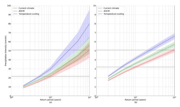
**Figure 4.** Intensity-duration-frequency (IDF) curves for current climate and future climate projected following Advanced Delta Change Method (ADCM) and the temperature scaling (a) 1-h events, and (b) 24-h events with 95% confidence interval indicated. The dashed lines represent the 10-year and 100-year precipitation intensities for the current climate.
