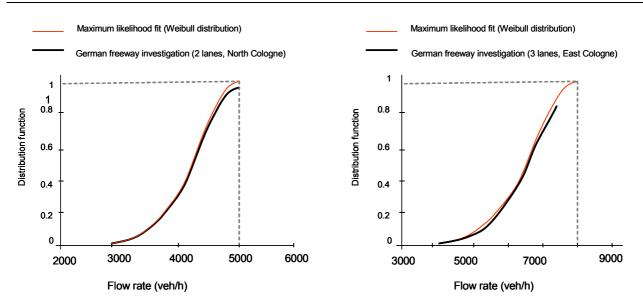
Figure 3.13: Capacity distribution functions for two German freeway sections - 5 min data
