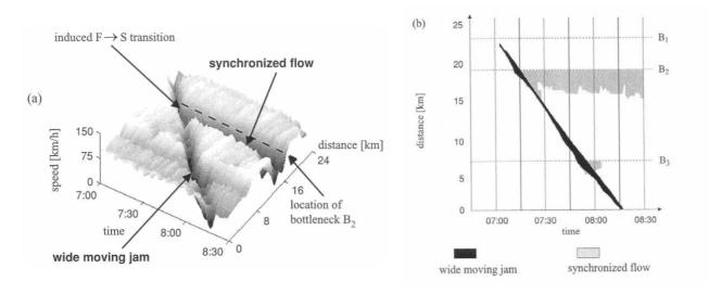
Figure 3.4: Synchronised flow and wide moving jams in congested traffic
