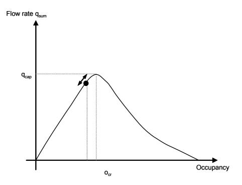
Figure 3.9: Fundamental diagram of free-flow control approach
