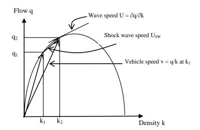
Figure 2.3: The relationship between vehicle speed, wave speed and shock wave speed
