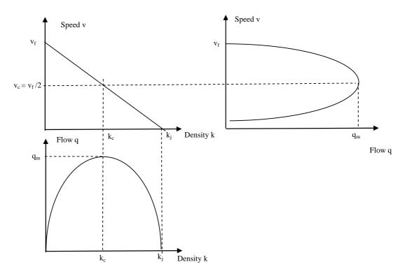
Figure 2.1: Fundamental diagrams assuming linear speed-density relationship
