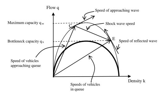
Figure 2.4: Fundamental diagrams of a bottleneck section and the approach section
