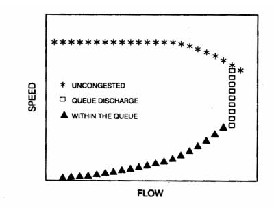
Figure 3.2: Generalised speed flow relation for a typical freeway segment
