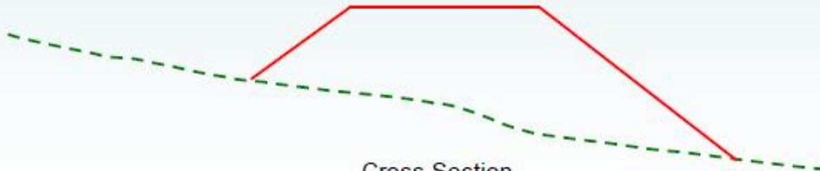
Cross Section Embankment (Fill)
