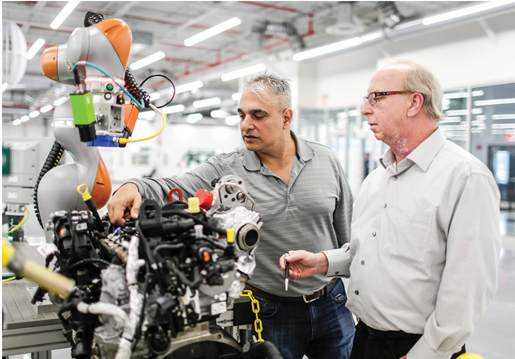
Harry Kekedjian (left) and Frank Maslar, Ford technical specialists, work with a collaborative robot, a smaller robot that can work safely alongside people without a protective cage.
