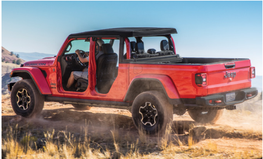
Based on the Wrangler SUV, but to accommodate a 5-ft cargo bed the Gladiator is some 31 in longer.
