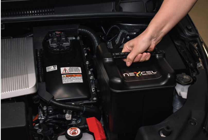
Extraction of the Nexcel module in the Toyota Prius demonstration vehicle.
