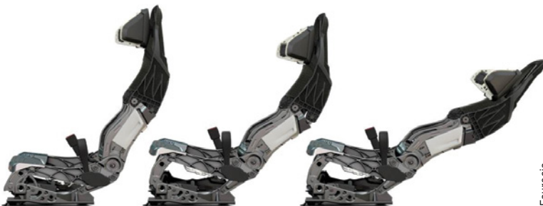
A Faurecia seat designed in conjunction with ZF embeds pyrotechnics in the frame, making it easier to return passengers to safe positions.
