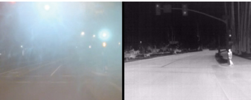
Oncoming headlight effect on visible and thermal camera comparison in nighttime foggy driving conditions.
