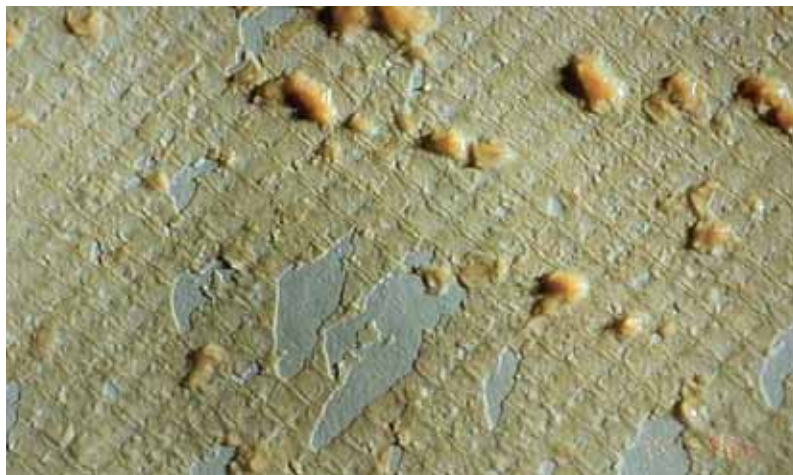
Figure 8.4 Picture of biofilm on membrane surface
