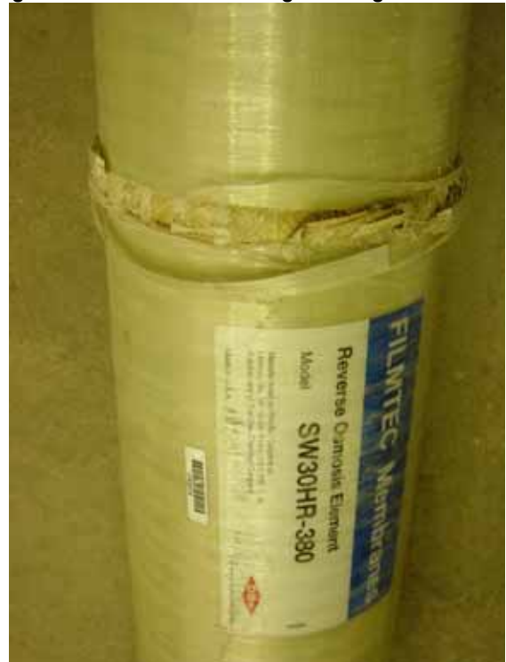
Figure 8.10 Picture of damaged fiberglass shell
