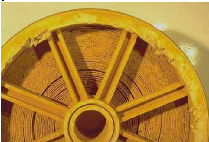
Figure 8.6 Picture of iron fouled feed side of an element with telescoping damage and signs of mechanical force
