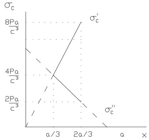
$$\frac{1}{3}a \leq x \leq \frac{2}{3}a \Rightarrow \sigma_{T \max} = \sigma''_T = \frac{12P(a-x)}{c^3} \leq \bar{\sigma} \Rightarrow c^3 \geq \frac{12P(a-x)}{\bar{\sigma}}$$
