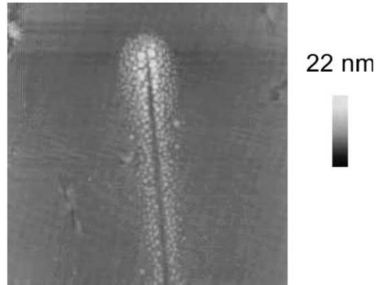
Fig. 7. Crystallites at the surface of glass close to the tip of an aged indentation crack. AFM view, size of field:  $8.5 \mu\text{m} \times 8.5 \mu\text{m}$  (from [19]).
