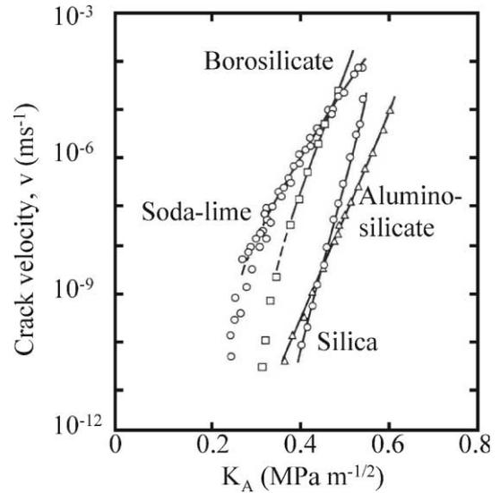
Fig. 3. Effect of glass composition (in water, from [25] after [9]).
