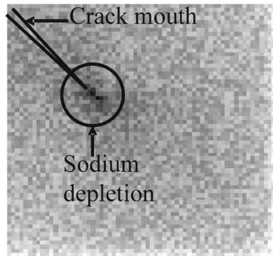
Fig. 8. EDX cartography of sodium close to the tip of an aged indentation crack. Top view, size of field:  $20 \mu\text{m} \times 20 \mu\text{m}$  (from [19]).
