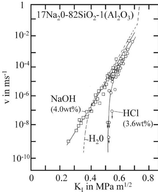
Fig. 4. Effect of an acid and of an alkaline medium on the crack growth (from [10]).
