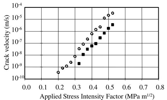
Fig. 6. Influence of the quality of annealing on the  $v-K_I$  curve obtained with DT test-samples. (○) as-float; residual core stress: 0.75 MPa, (■) special annealing, residual core stress 0.25 MPa).
