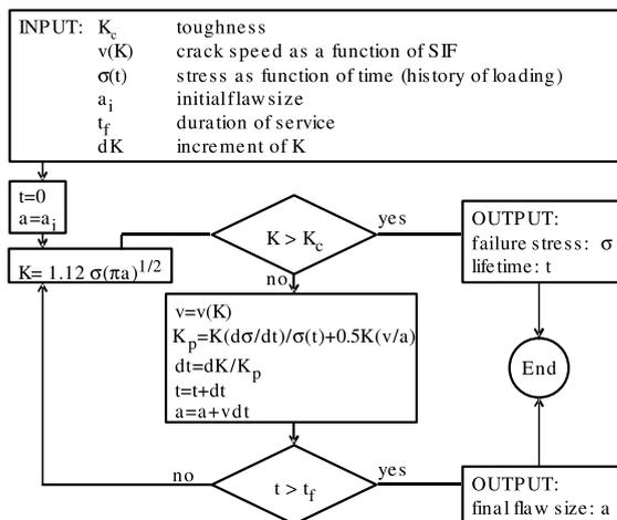
Fig. 5. Numerical procedure for the computation of time to failure for a glass body with a small straight surface crack under uniform far field stress, for any given  $v-K_I$  curve, and any given loading history.
