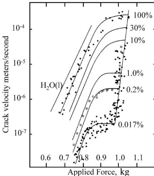
Fig. 2. Effect of an increasing amount of water in the environment (from [7]).
