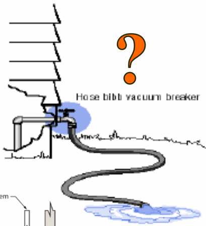
Typical installation of hose bibb vacuum breaker.
