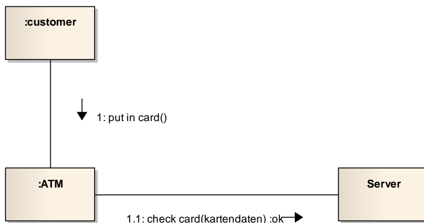
Fig. 56: Example of the “Identify Authorization” Communication Diagram
