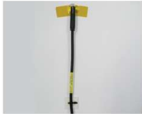
The 110PV is mounted to the measurement surface via Kapton tape.
