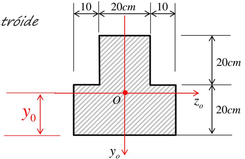
$$y_o = \frac{40 \times 40 \times 20 - 2 \times 10 \times 20 \times 30}{40 \times 40 - 2 \times 10 \times 20}$$
