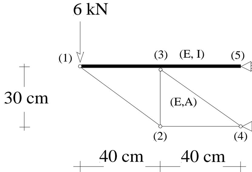
Resp.:  $N_{12} = -10,0 \text{ kN}$ ;  $N_{23} = 6,0 \text{ kN}$ ;  $N_{34} = -10,0 \text{ kN}$ ;  $N_{24} = -8,0 \text{ kN}$ .
