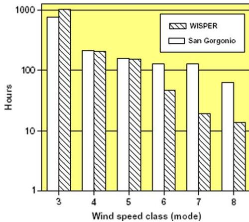
Fig. 10. Wind speed distributions according to WISPER and measurements at a Californian site [44].
