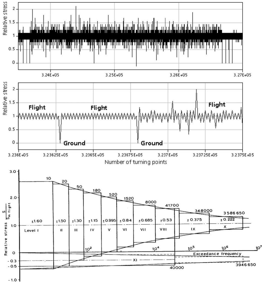
Fig. 12. Samples of the TWIST load sequence (top) and the TWIST spectrum (40,000 flights) consisting of gust, ground-air-ground and taxiing load elements (bottom).
