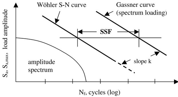
Fig. 2. Wöhler and Gassner S–N curves and the factor SSF.
