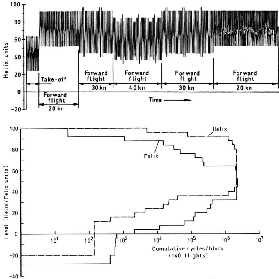
Fig. 6. Example of HELIX, first phase of a training flight (top) and level cross spectra of FELIX and HELIX (bottom).
