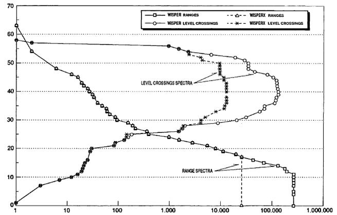
Fig. 9. Level crossing and rainflow (ranges) spectra of WISPER.
