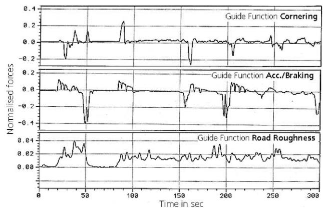
Fig. 7. Guide functions (CARLOS multi): e.g. cornering, sum of front lateral forces.
