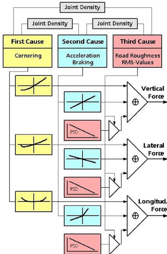
Fig. 8. Guide function approach for synthesis of partly correlated multiaxial load–time histories, car wheel suspension [23]; PSD, power spectral density.
