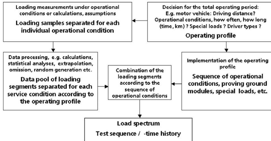
Fig. 4. General (simplified) approach for the generation of SLH's (example: passenger vehicle).
