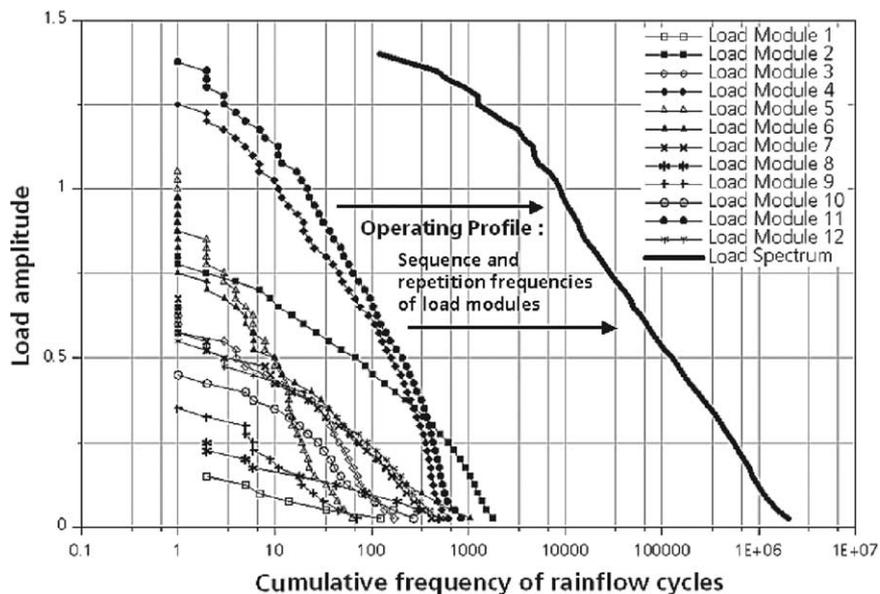
Fig. 5. Compilation of a load spectrum by simple repetition of loading segments according to the associated operating profile.
