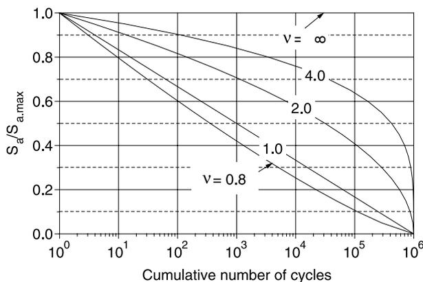
Fig. 3. Typical load amplitude spectra.
