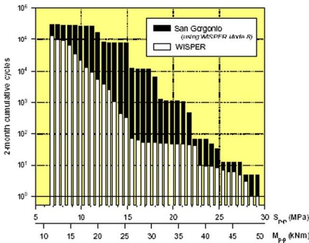
Fig. 11. Comparison of the WISPER spectrum and a 2-month spectrum derived on wind measurements and the WISPER protocol [44].
