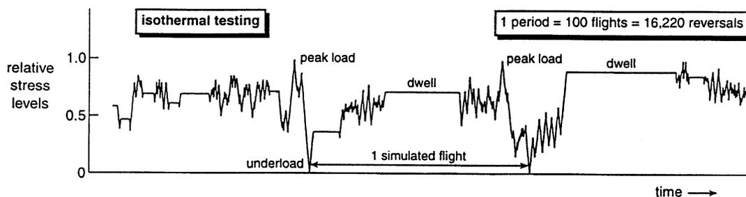
Fig. 1. Segments of Hot TURBISTAN, load reversals plus dwell times.
