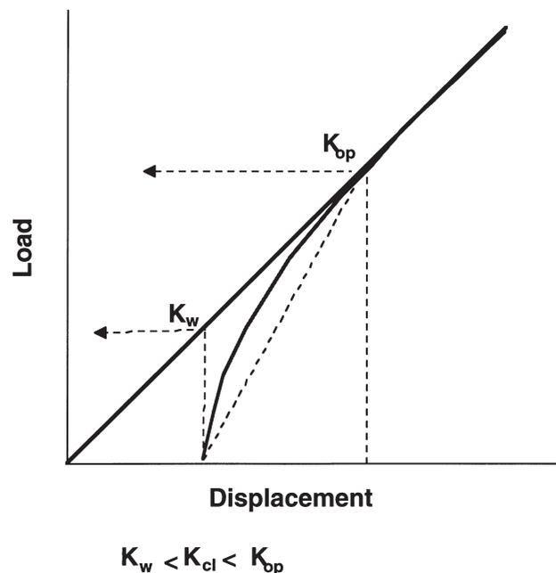
Fig. 2. Load-Displacement curve and corrected crack closure measurement (CCCM) using the load-displacement curve.
