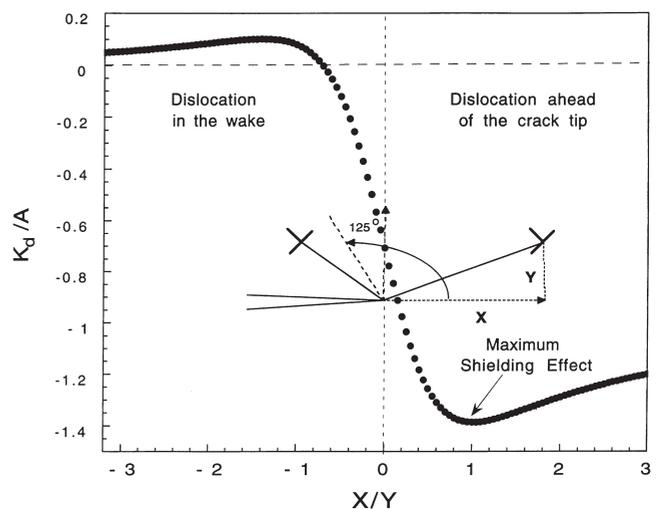
Fig. 13. Shielding effect of a dislocation ahead of the crack tip showing that maximum compression force occurs not at the crack tip but at a distance from the crack tip.
