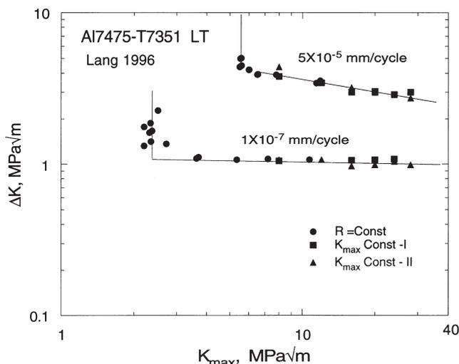
Fig. 4. Log–log plot of the data in Fig. 3 to show the exponential dependence on  $K_{max}$  at high  $R$  values.
