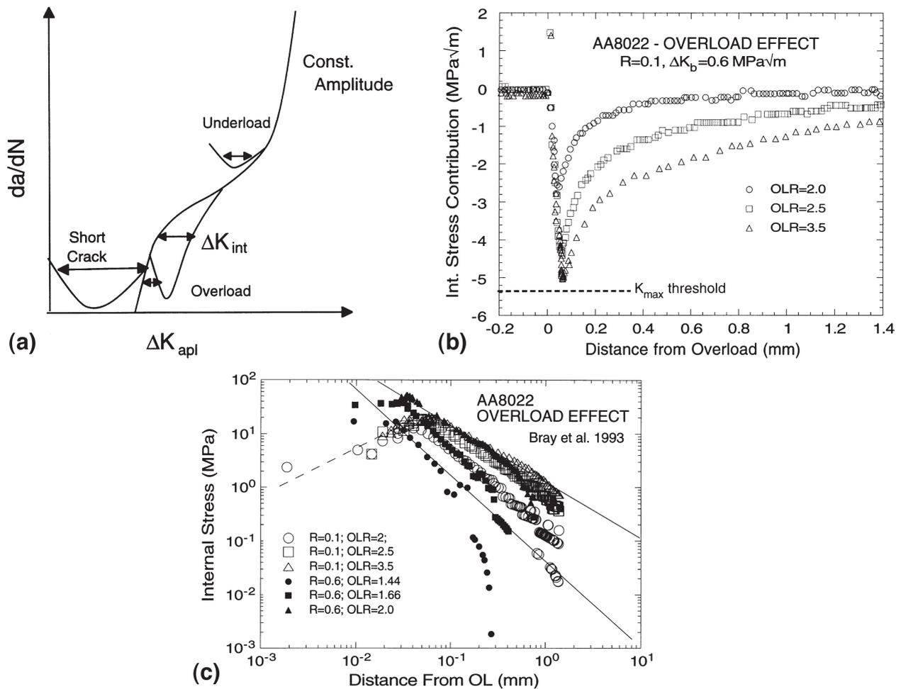
Fig. 12. (a) Schematic illustration for extracting internal or residual stresses from  $da/dN$  curves. (b) The residual stress profile as a function of incremental crack length for an AA8022 Aluminum alloy. (c) Residual or internal stresses as a function of crack increment on a log-log scale.
