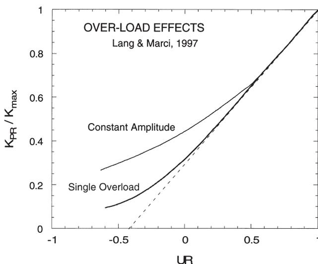
Fig. 9. Effect of overload on  $K_{pr}$  in comparison to its steady state  $K_{pr}$  value.
