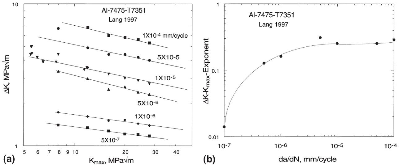
Fig. 5. (a) The exponential dependence is a function of crack growth rate. (b) The variation of the exponent with crack growth rate.
