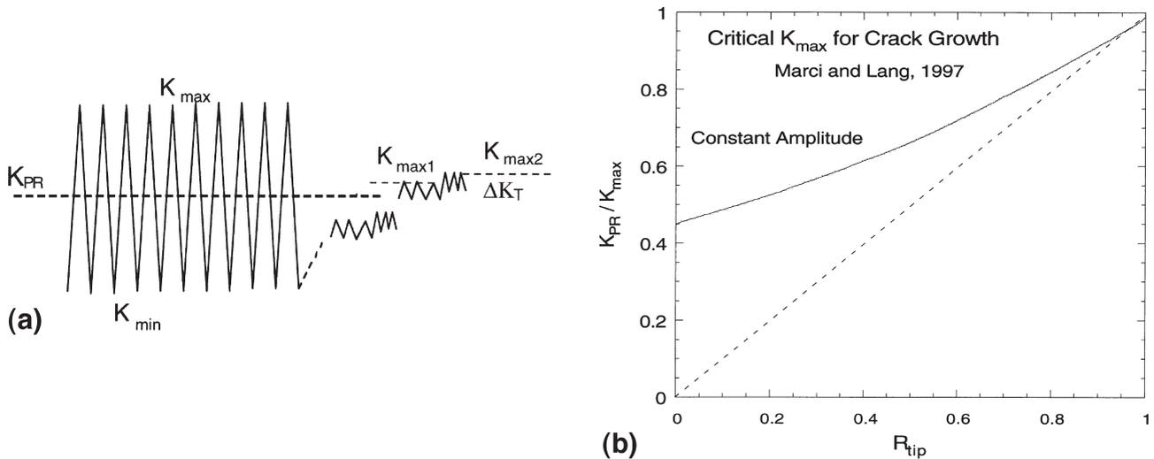
Fig. 6. Schematic illustration of the experimental determination of  $K_{pr}$  using Crack Propagation Load Measurement (CPLM) by Lang and Marci. (b) Variation of  $K_{pr}$  with  $R_{tip}$  where  $R_{tip}$  is the  $R$ -value corrected for crack closure.
