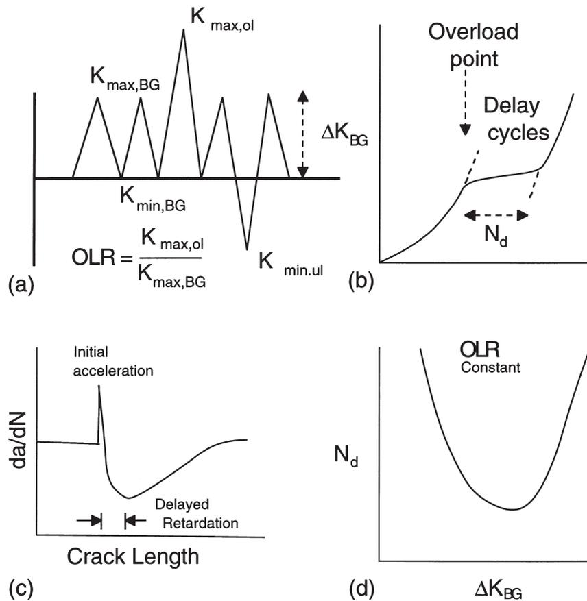
Fig. 1. Schematic illustration of the overload effects on fatigue crack growth.
