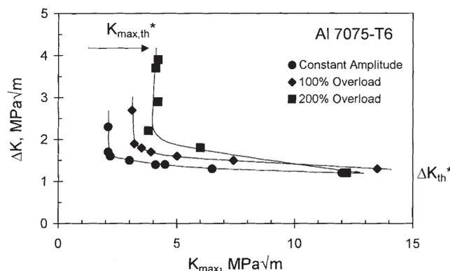
Fig. 11. Independent evaluation of overload effects on the  $\Delta K$ - $K_{\max}$  curve for a Al-7075-T6 alloy at two overload ratios. The curves shift to the right as illustrated in Fig. 10.
