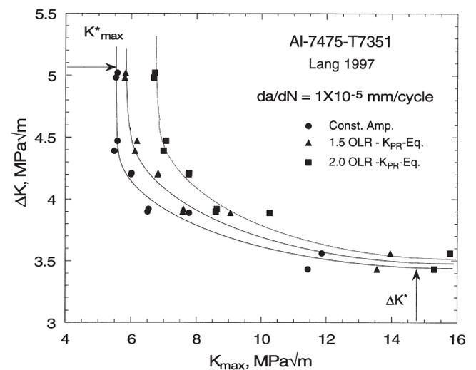
Fig. 10. Demonstration of how overload  $K_{pr}$  affects  $\Delta K - K_{max}$  curves by shifting the curves to the right due to the compressive residual stresses affecting crack tip driving force,  $K_{max}$ . Equivalence of the two approaches is shown.
