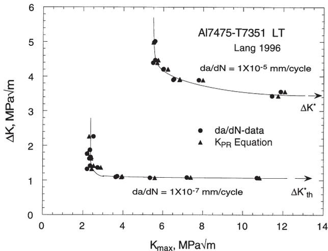
Fig. 7. Identity of  $\Delta K$ – $K_{\max}$  extracted from the raw  $da/dN$  data and that from the empirical equation of  $K_{pr}$  determined independently by CPLM method. Experimental  $K_{pr}$  confirms independently the critical  $K_{\max}$  required for crack growth and its relation to crack tip plasticity ahead of the crack tip.
