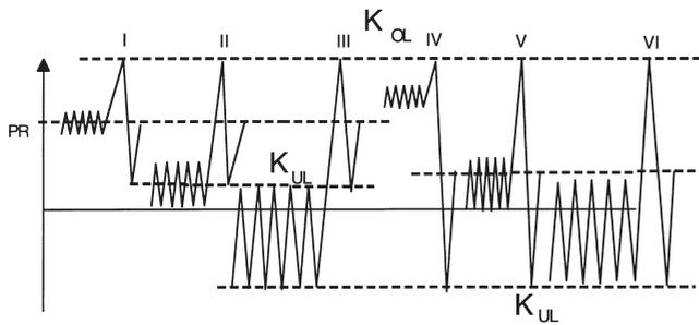
Fig. 8. Schematic illustration of  $K_{pr}$  for overload and under loads and its dependence on the  $K$  values at the spike loads, from Lang and Marci.
