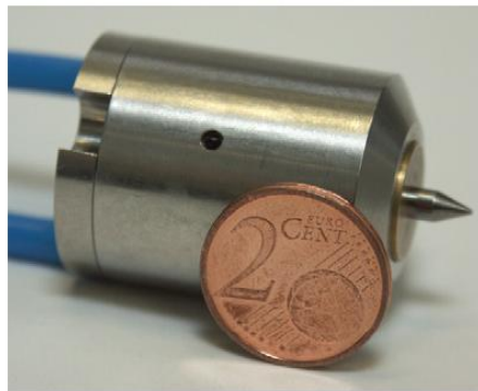
Fig. 5. High speed air bearing spindle.
