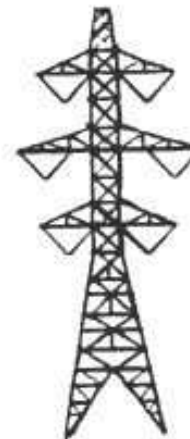
500 kV Steel Lattice Double Circuit Average height 170' Average span 1150'
