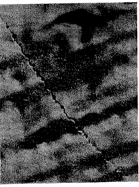
Fig. 11. Aluminum-2% magnesium alloy tested in creep rupture at 500°F and 4000 psi. Rupture life, 5 hr. Stress direction is vertical.
