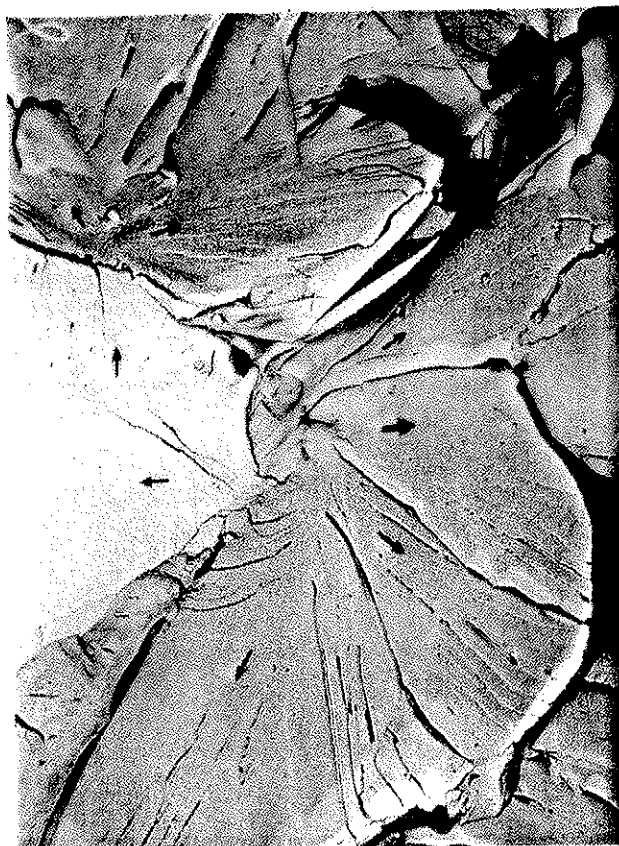
Fig. 11. Example of distorted region at grain boundary between cleaved grains in polycrystalline iron deformed 7.5% in bending at 78°K.
