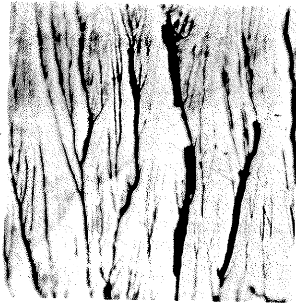
Fig. 1. Cleavage step "river pattern." 3% Si-Fe single-crystal cleavage surface. Cleaved at 78°K. Direction of crack propagation is from top to bottom of the photograph. Note low-angle tilt boundary.
