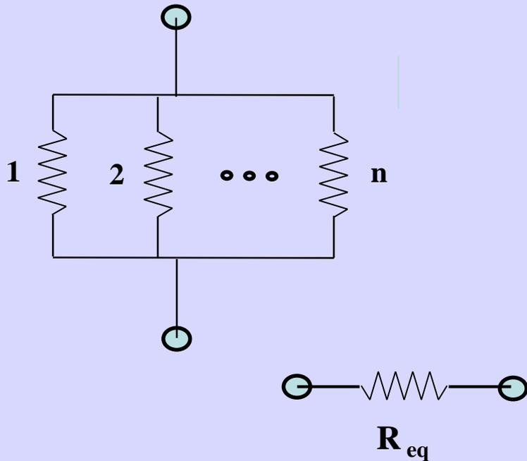
$$\frac{1}{R_{eq}} = \frac{1}{R_1} + \frac{1}{R_2} + \dots + \frac{1}{R_n}$$
