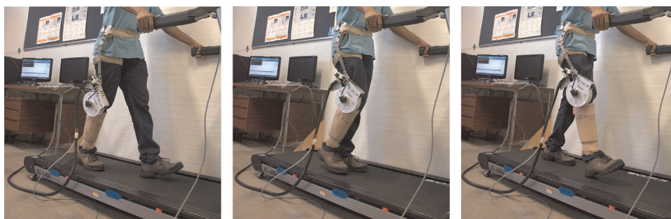
Fig. 8. Rotary SEA attached to a knee orthosis.
