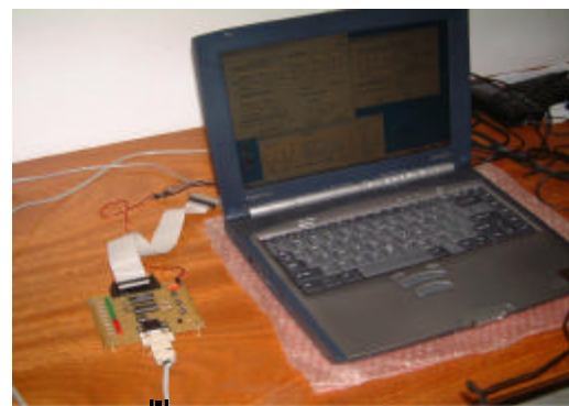
Figura 8.3-Conexão PC transmissor com PC receptor
