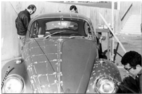
A Volkswagen Beetle becomes the subject of a 1970 simulation project. Ivan Sutherland(left) and assistants plot coordinates for digitizing the car.
