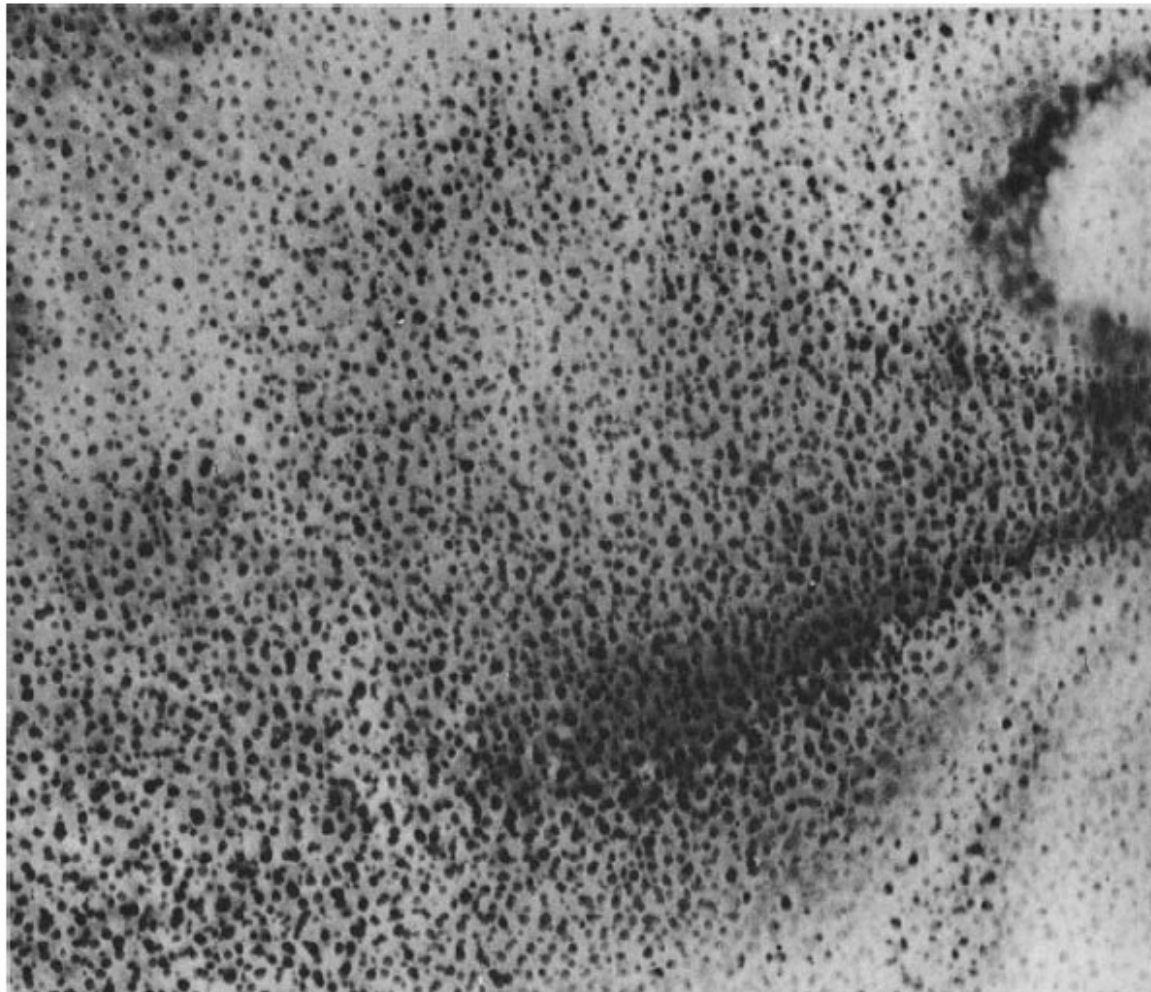
FIG. 16.8 Guinier-Preston zones in an aluminum 16 percent silver alloy. (Reprinted from Nicholson, R.B., and Nutting, J., Acta. Met. 9 332 [1961] with permission of Elsevier. Photograph courtesy of RB Nicholson. http://www.sciencedirect.com/science/journal/00016160 )
