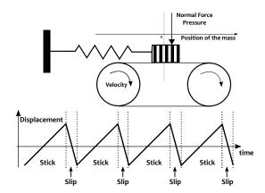
Figure 3: The Conveyer-Belt Model and a Typical Stick-Slip Mo-
