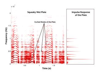
Figure 5: Squeaky Wet Plate and its Impuse Response
