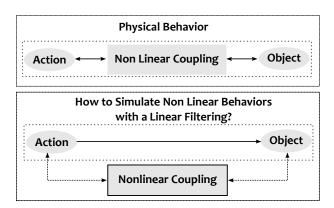
Figure 2: How to Separate the Non Linear Coupling to Implement Non Linear Behaviors with Linear Filtering
