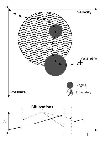
Figure 7: An Example of Control Strategy by Defining the Vibrating Behavior According to Velocity / Pressure Areas and the Mapping Function Between the Descriptors  $\gamma$  and the Fundamental Frequency  $f_0$
