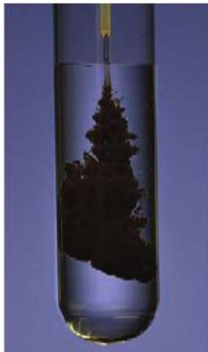
**(b)**  $\text{Pb}(\text{NO}_3)_2$  and  $(\text{NH}_4)_2\text{S}$  produce black, insoluble  $\text{PbS}$  and soluble  $\text{NH}_4\text{NO}_3$ .
