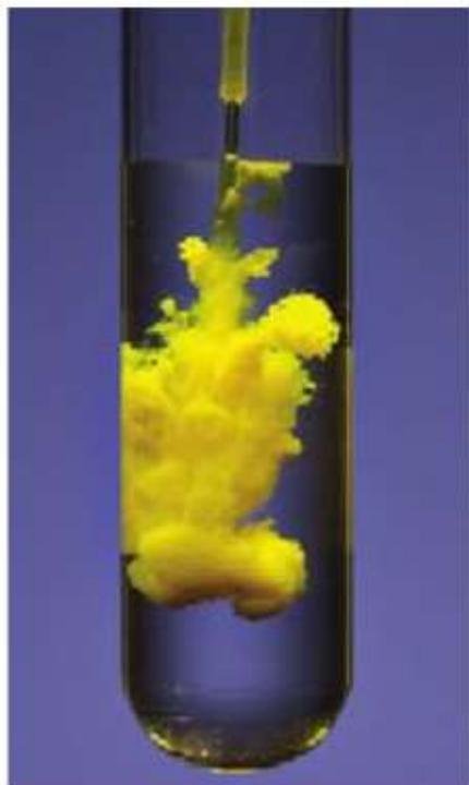
**(a)**  $\text{Pb}(\text{NO}_3)_2$  and  $\text{K}_2\text{CrO}_4$  produce yellow, insoluble  $\text{PbCrO}_4$  and soluble  $\text{KNO}_3$ .
