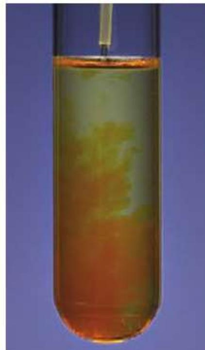
**(c)**  $\text{FeCl}_3$  and  $\text{NaOH}$  produce red, insoluble  $\text{Fe}(\text{OH})_3$  and soluble  $\text{NaCl}$ .
