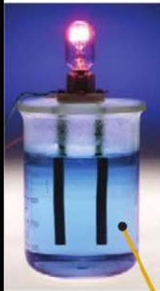
A **strong electrolyte** conducts electricity.  $\text{CuCl}_2$  is completely dissociated into  $\text{Cu}^{2+}$  and  $\text{Cl}^-$  ions.
