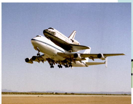
Dryden Flight Research Center EC96-43518-1 Photographed 4/96 Shuttle STS-76 is transported to Kennedy Space Center in Florida by a NASA 747 after landing at Dryden. NASA Photo
