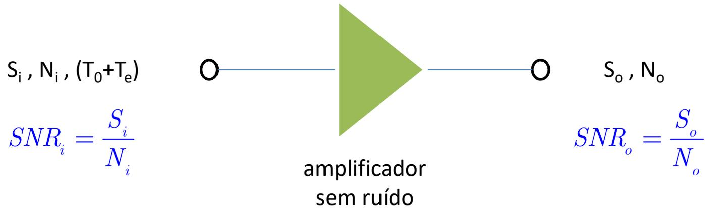
$$SNR_i = \frac{S_i}{N_i} = \frac{S_i}{KT_o B} \qquad SNR_o = \frac{S_o}{N_o} = \frac{S_o}{G_A K (T_o + T_e) B}$$
