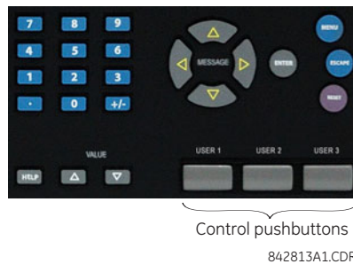
Figure 5-33: Control pushbuttons (enhanced faceplate)
