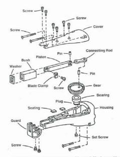
Figure 3.14 Power saw (new design-29 parts, 2.58 min assembly time). (After Ref.
