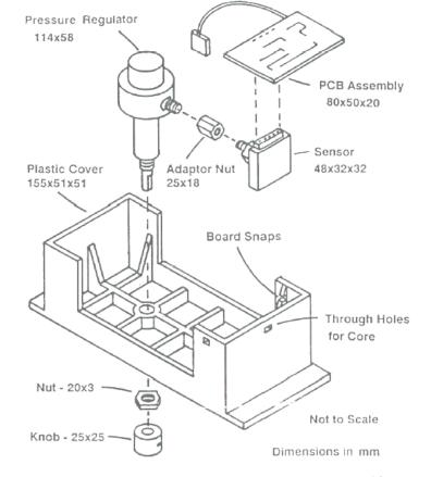
Figure 3.37 Conceptual redesign of the controller assembly.
