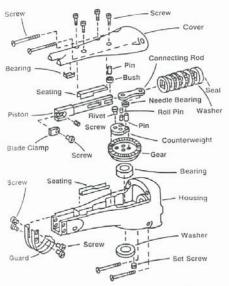
Figure 3.13 Power saw (initial design-41 parts, 6.37 min assembly time). (After Ref. 14.)
