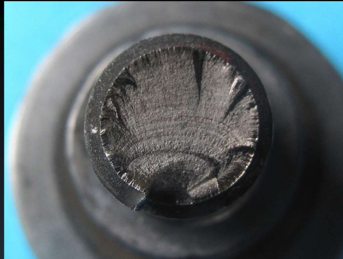
Fractograph of fatigue failure in SAE 1050 pin, induction hardened to a depth of 5 mm (3/16 in.) and surface hardness of 55 HRC. Core hardness: 21 HRC. Fatigue initiated inside the grease hole at the metallurgical notch created by the very sharp case-core hardness gradient.
