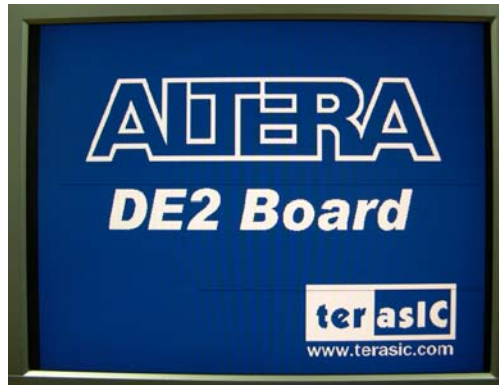
Figure 2.3. The default VGA output pattern.
