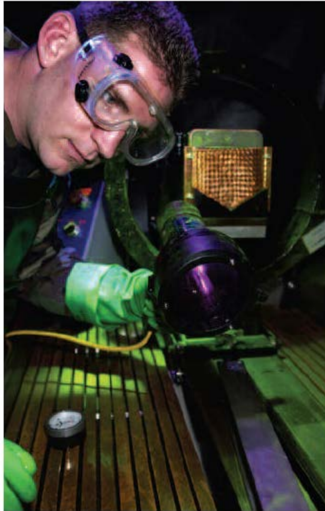
Figure 4. An Inspector Performing a Magnetic Particle Inspection of a Component.
