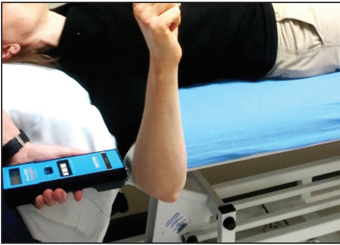
Figure 2. Abduction strength measurement with dynamometer
