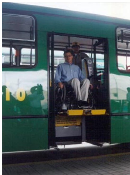
Fig. 13.79 A special lift allows access for a wheelchair patron to a high-floor feeder vehicle in Bogotá.
