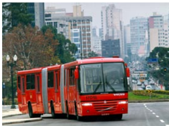
Fig. 12.3 In Curitiba, 24-metre bi-articulated vehicles are utilised on trunk corridors. Photo courtesy of Volvo Bus Corporation
