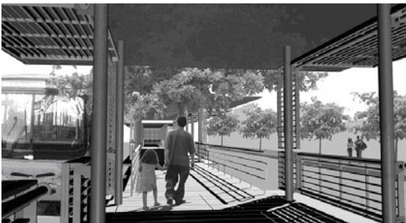
Fig. 11.58 Passive solar design provides shading and encourages natural air flows without the need for costly air conditioning systems.
