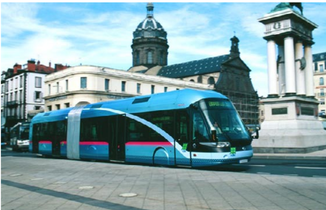
Fig. 2.55 Modern vehicles can give BRT systems a highly professional image. The vehicle in this photo is a Cibus bus and not a light rail vehicle.
