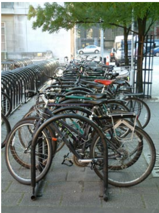
Fig. 13.95 A self-locking U shaped post is a low-cost and relatively secure option. Photo by Lloyd Wright
