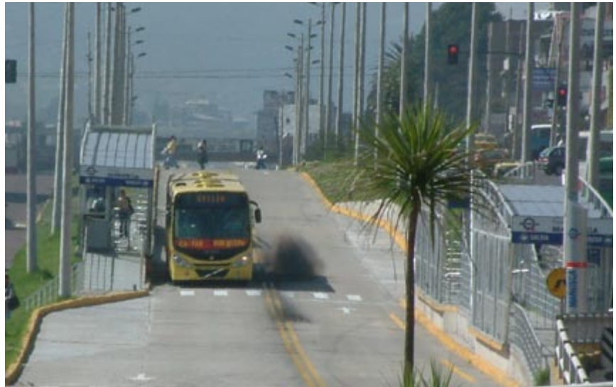
Fig. 12.25 On the Quito Central Norte corridor, the Euro III compliant vehicles are not producing the desired results due to the use of 500 ppm diesel fuel.
