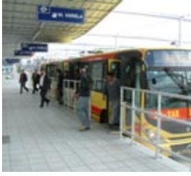
Fig. 10 At-level platforms provide rapid boarding and alighting in Quito. Photo by Lloyd Wright
