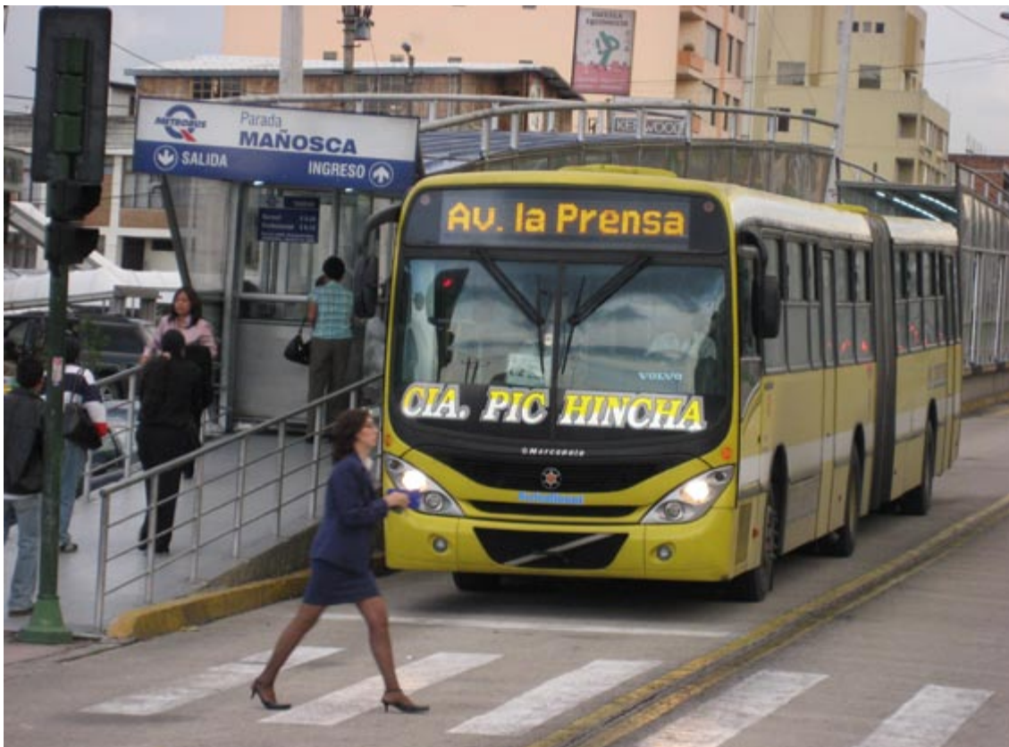
Fig. 13.43 Due to their ease of use and directness, at-grade crossings are almost always the preference of customers.
