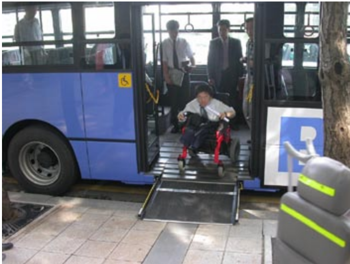
Fig. 13.77 A manually operated ramp extended from the bus provides access for wheelchair users.
