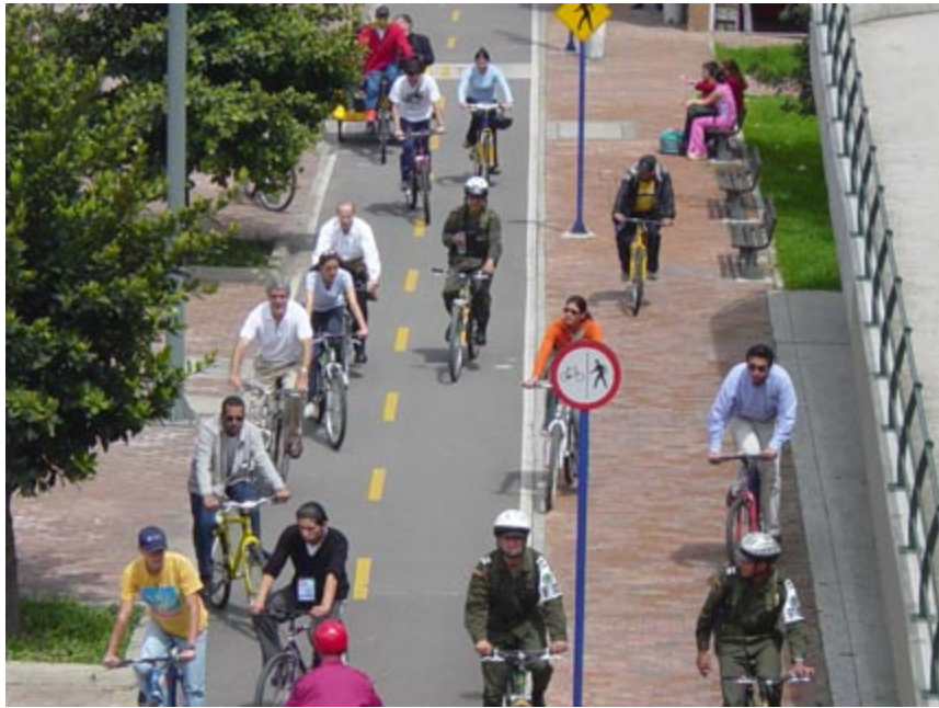
Fig. 13.103 Wide cycleways and footpaths allow the two modes to be successfully integrated in Bogotá.
