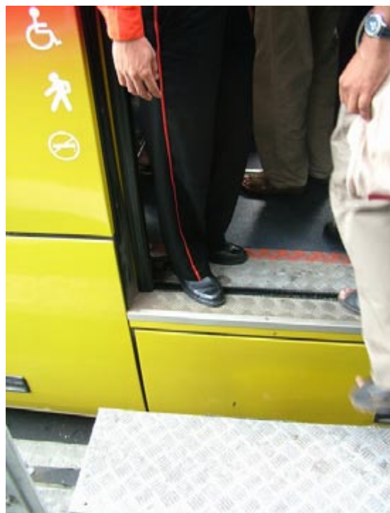
Fig. 8.26 The substantial gap between the vehicle and platform in Jakarta can be a significant safety risk to customers.
