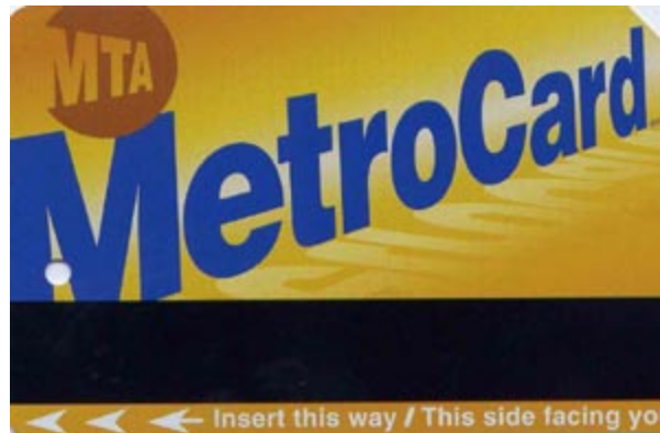
Fig. 12.56 and 12.57 There are two types of magnetic strip cards: 1. The standard sized card, as shown in this example from the New York subway (left image); and, 2. The smaller Edmonson card, as shown in this example from the Paris Metro (right image).
