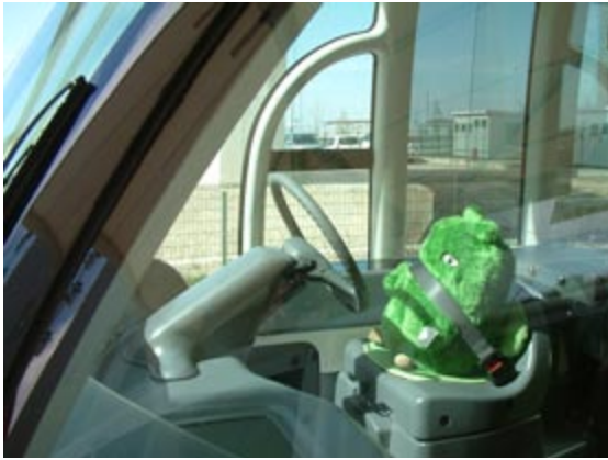
Fig. 18.3 In Aichi (Japan), a toy mascot is given the driver's seat in a driverless bus system with full optical guidance.
