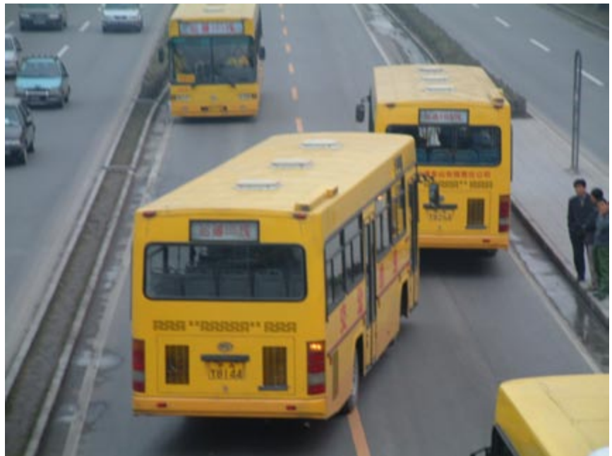
Fig. 7.31 By allowing vehicles to overtake in the opposing lane, there are obvious risks of a serious collision as evidenced in Beijing.
