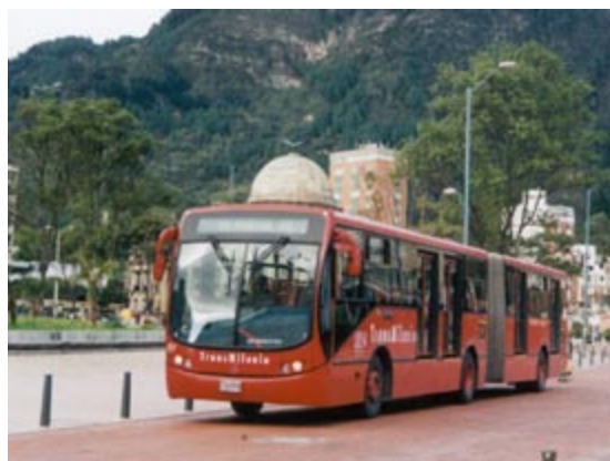
Fig. 12.4 In Bogota, 18-metre articulated vehicles are utilised. Photo courtesy of TransMilenio SA
