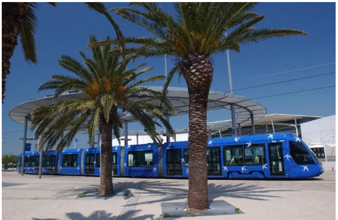
Fig. 2.40 For cities such as Montpellier (France), LRT provides a good public image and can adeptly serve moderate peak demands (less than 12,000 pphpd). Photo courtesy of UITP
