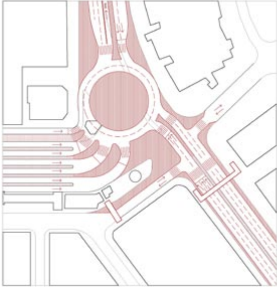
Fig. 13.15 A design was developed with multiple pedestrian islands in order to improve conditions. Image courtesy of Michael King
