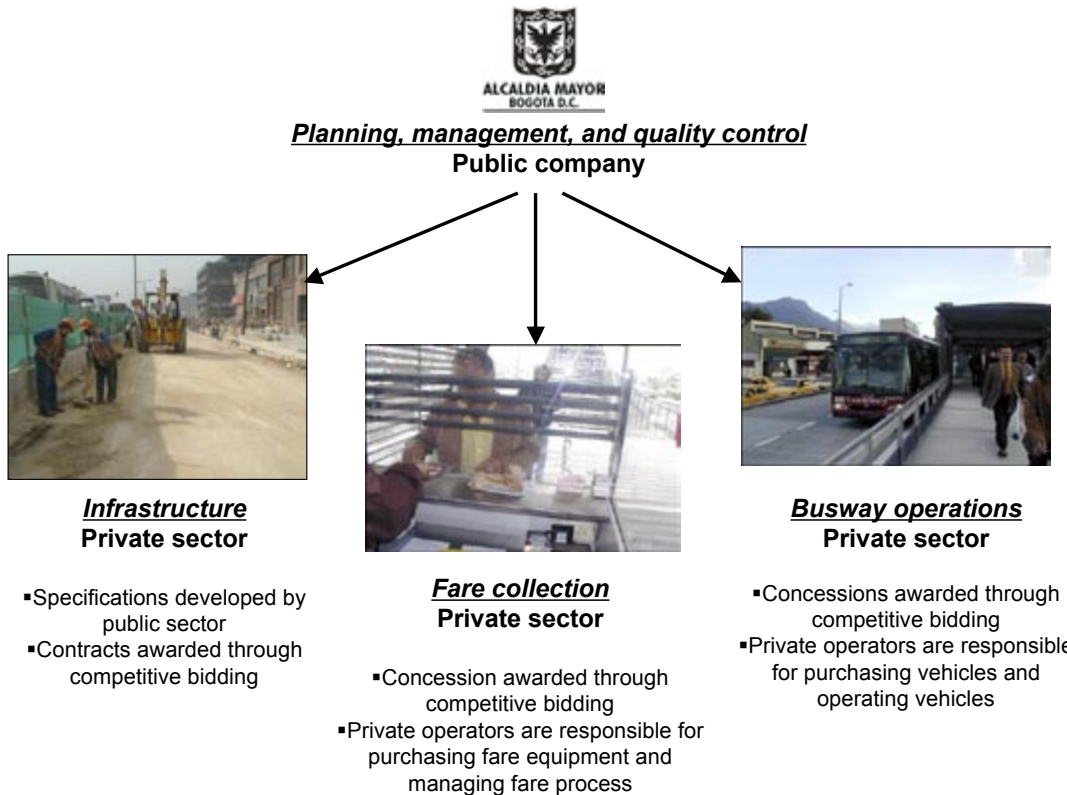
Fig. 15.16 The TransMilenio business structure features a public company overseeing quality control and contract management with an array of privately concessioned firms. Image courtesy of TransMilenio SA
