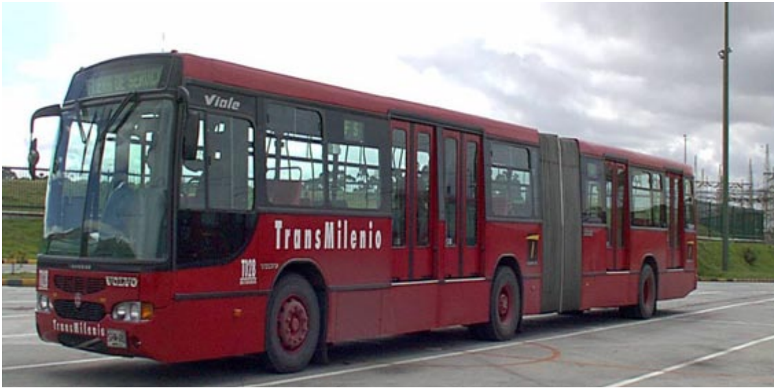
Fig. 12.18 Bogotá utilises a four door configuration that helps to reduce boarding and alighting times. Photo courtesy of TransMilenio TM
