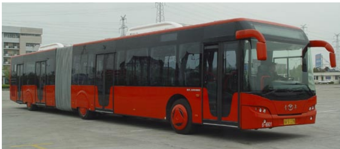
Fig. 8.12 The 18.5-metre articulated vehicle has become standard in many BRT applications.
