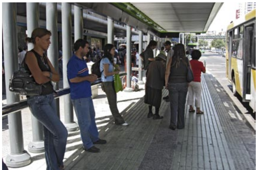
Fig. 11.72 A leaning post can be an economical way of providing comfort to waiting passengers.
