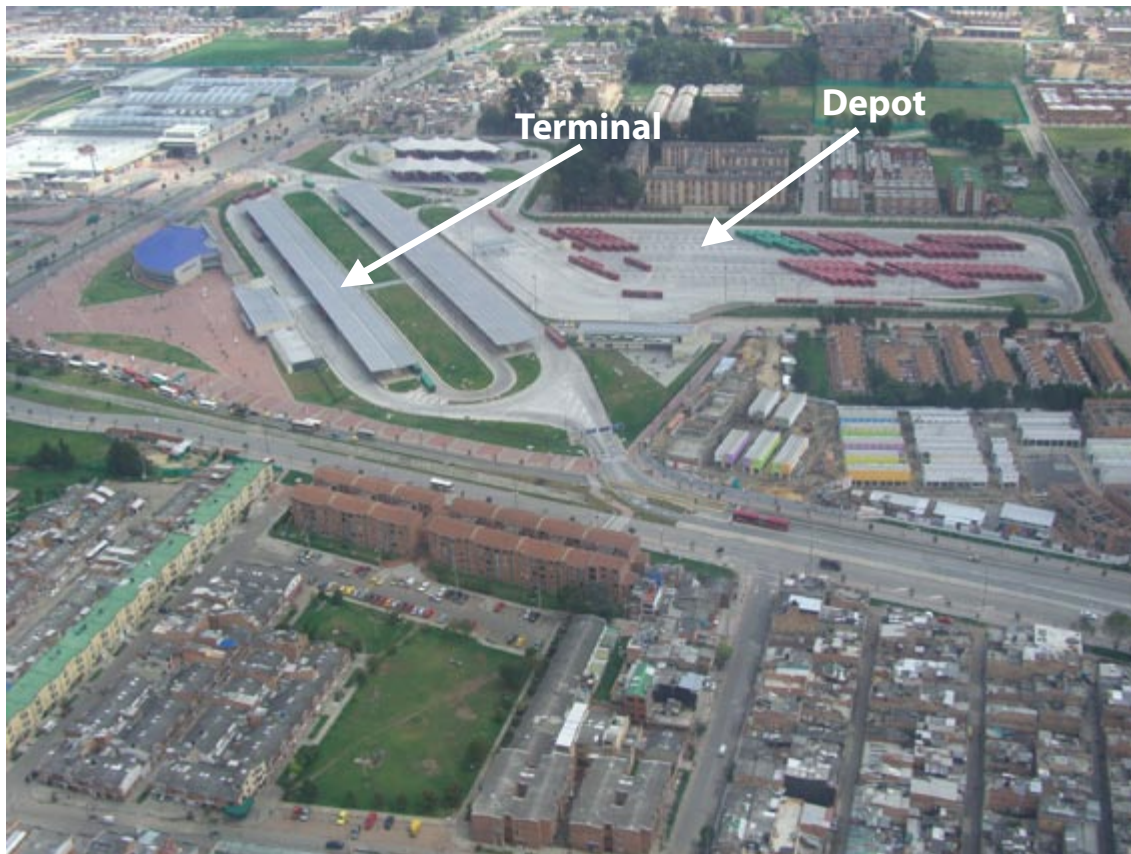
Fig. 11.102 In Bogotá, most depots are located next to the terminal areas in order to improve operational efficiency.
