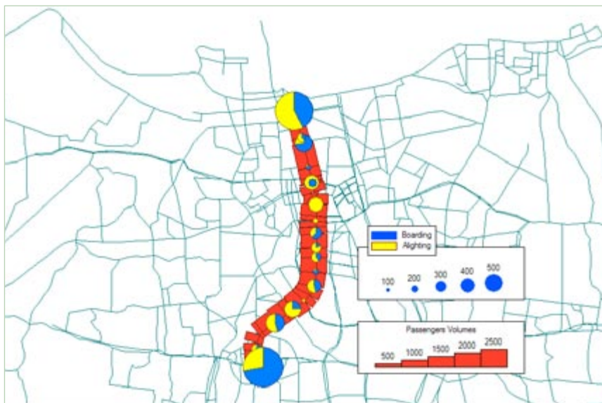
Fig. 4.25 Demand estimate for TransJakarta Corridor I, Scenario I. Image courtesy of ITDP
