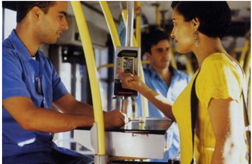
Fig. 8.19 In Brazil, a “reservoir” space is provided within the vehicle where passengers queue to verify their fare. With the use of this reservoir, the vehicle is able to proceed even before all passengers have verified their fare.
