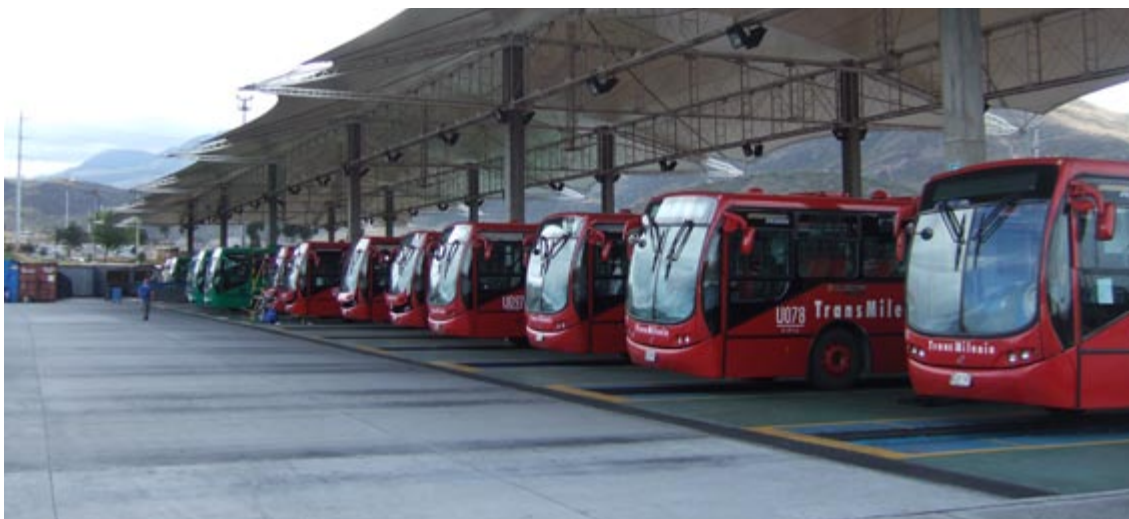
Fig. 8.14 The size of the required vehicle fleet demands on corridor demand, travel time to complete a corridor cycle, and each vehicle’s passenger capacity. Photo by Lloyd Wright
