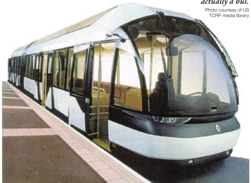
Fig. 12.39 Despite giving a distinctly light rail appearance, the Cavis vehicle is actually a bus.
