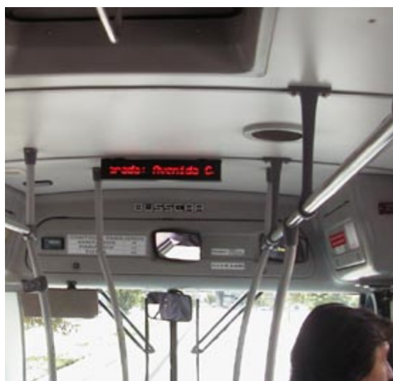
Fig. 10.16 An information display in the interior of a TransMilenio vehicle in Bogotá.
