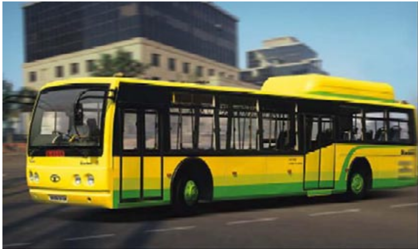
Fig. 12.9 A new CNG modelled low-floor vehicle developed by Tata Motors for the Dehli BRT system.
