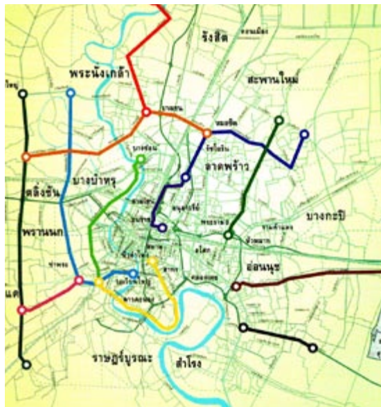
Fig. 3.23 The proposed Bangkok BRT system of the Bangkok Metropolitan Administration (BMA) features a corridor plan that forces all customers to transfer to other modes prior to arriving in the city centre.
