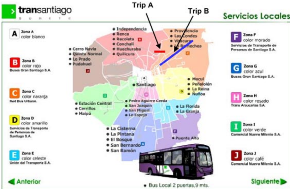
Fig. 16.20 In this example from Santiago, the short passenger trip (Trip A) will cost double the long passenger trip (Trip B). Zonal fare systems can thus provide simplicity at the expense of fare equity.
