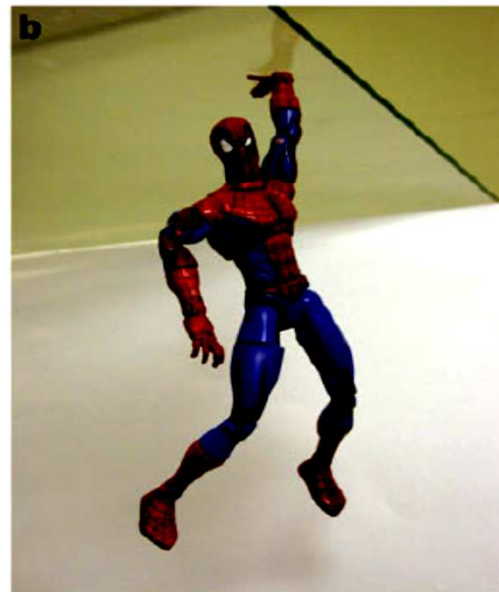
Fig. 11.29 (a) (left) An array of polyimide nanohairs and (right) bunching of the nanohairs, which leads to a reduction in adhesive force. (b) A Spiderman toy (about 0.4 N) with a hand covered with the molded polymer nanohairs, clinging to a glass plate (Geim et al., 2003)
