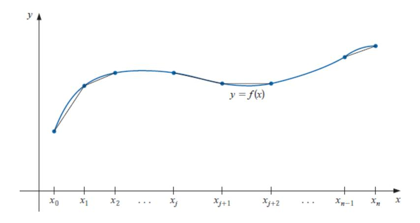
A disadvantage of linear function approximation is that there is likely no differentiability at the endpoints of the subintervals, which, in a geometrical context, means that the interpolating function is not "smooth." Often it is clear from physical conditions that smoothness is required, so the approximating function must be continuously differentiable.
