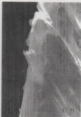
Figure 14.13 SEM of extrusions and intrusions in a copper sheet. (Courtesy of M. Judelwicz and B. Ilchner)
