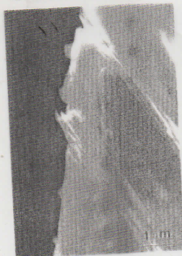
Figure 14.10 (a) Persistent slip bands in vein structure. Polycrystalline copper fatigued at a total strain amplitude of 6.4 \times 10^{-4} for 3 \times 10^5 cycles. Fatiguing carried out in reverse bending at room temperature and at a frequency of 17 Hz. The thin foil was taken 73 \mu\text{m} below the surface. (Courtesy of J. R. Weertman and H. Shirai) (b) Cyclic stress-strain curve for a single crystal of copper oriented for single slip (After H. Mughrabi, Mater. Sci. & Eng. 33 (1978) 707).
