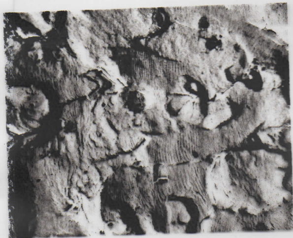
Fig. 15. Microfractograph of a fatigue rupture surface of duralumin (alternate bending, \pm 7 kg/mm 2 , rupture in 0.27 \times 10^6 cycles).
