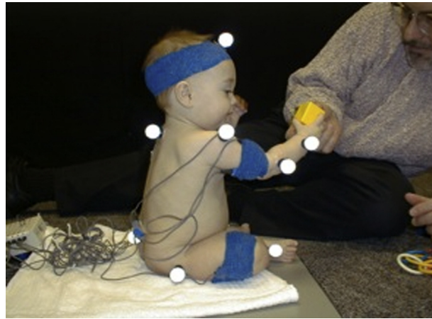
Fig. 1. Infant prepared for data collection. Markers for body segment measurement with the VICON system appear as lighted spheres.
