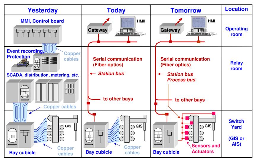
*Functionality:* SA to control,operate, monitor, and protect the substation
