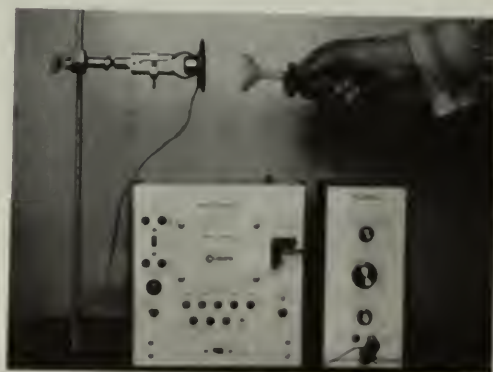
Fig. 3-61 Sound from the speaker can be detected by using a funnel and rubber hose, the end of which is placed to the ear. The oscillator's banana plug jacks must be inserted into the -8 V, +8 V, and ground holes of the power supply. Insert the speaker's plugs into the sine wave ground receptacles of the oscillator. Select the audio range by means of the top knob of the oscillator and then turn on the power supply.
