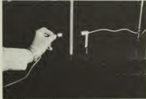
Fig. 3-66 Detecting diffraction of ultrasound around a barrier.
