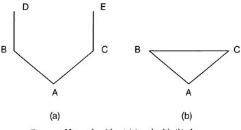
FIG. 1.—Network without (a) and with (b) closure
