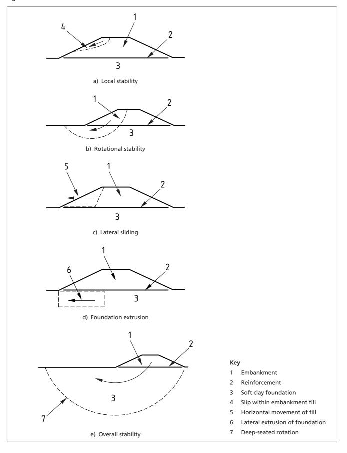
Figure 70 Serviceability limit states for basal reinforced embankments
