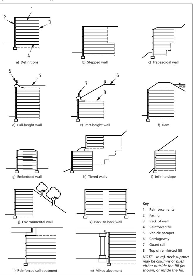
Figure 16 Common facings used with structures
