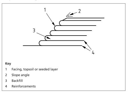
Figure 64 Wrap-around construction techniques
