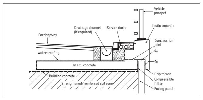
Figure E.6 Illustrative detail of a parapet-supporting base slab at the top of a strengthened/reinforced soil wall with pre-cast concrete coping
