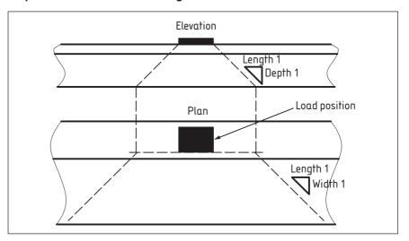
Figure E.3 Distribution of pressure beneath a base slab
