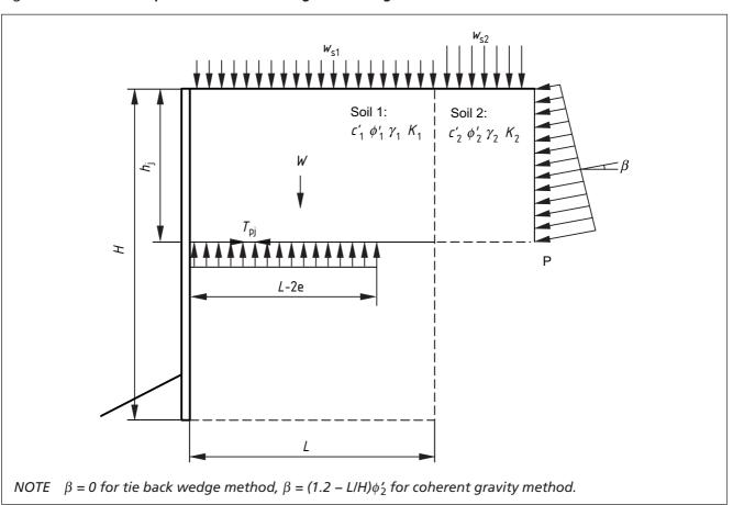
Figure 29 **Dispersal of vertical strip load through reinforced fill – Tie back** wedge method
