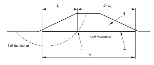
b) Reinforcement bond lengths at position j along base of embankment
