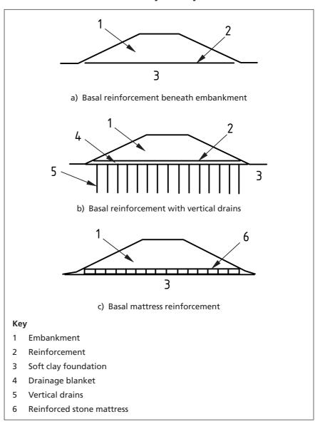
Figure 68 Reinforcement used to control both stability and settlement of embankment
