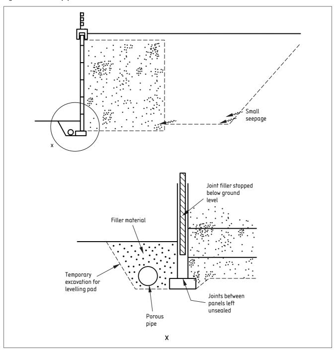
Figure 51 Drainage details for walls supporting cuttings
