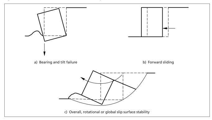
Figure 23 Seviceability limit states – External and internal stability
