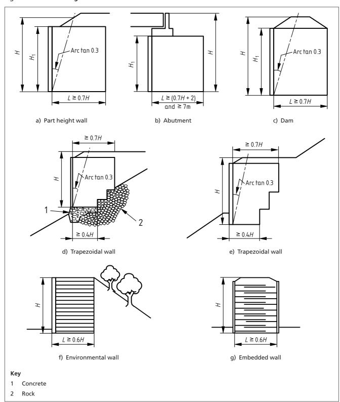
Figure 20 Sizing of walls with various geometries
