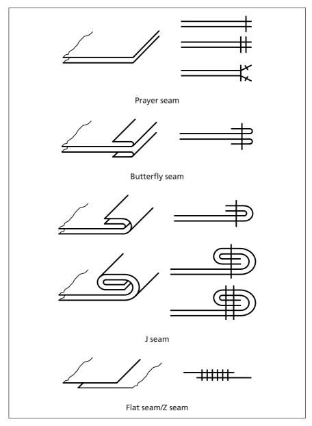
Joints should be formed to have the highest mechanical and durability efficiency possible, compared to the performance characteristics of the parent materials. Test methods used to assess joints should correspond closely to those procedures employed when determining the properties of the parent materials. All joints used in permanent structures designed to carry loads should be tested in accordance with BS EN ISO 10321.
