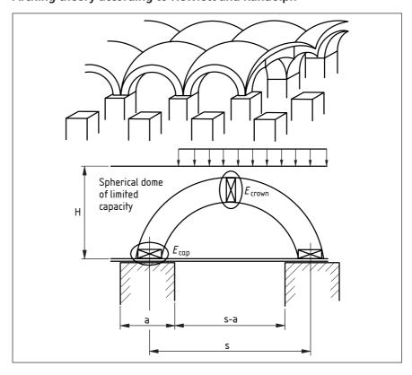
The proportion of embankment weight supported directly by the piles may be determined from.
