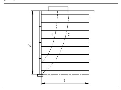
Figure 41 Definition of line 1 – Coherent gravity method
