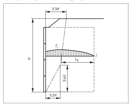
Figure 40 Lines of maximum tension for structures with strip loads – Coherent gravity method
