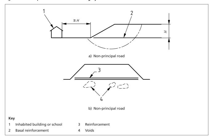
Figure 13 Examples of structures in category 3 – Applicable to walls and slopes
