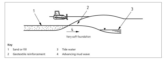
Figure 88 Inverted "U" construction
