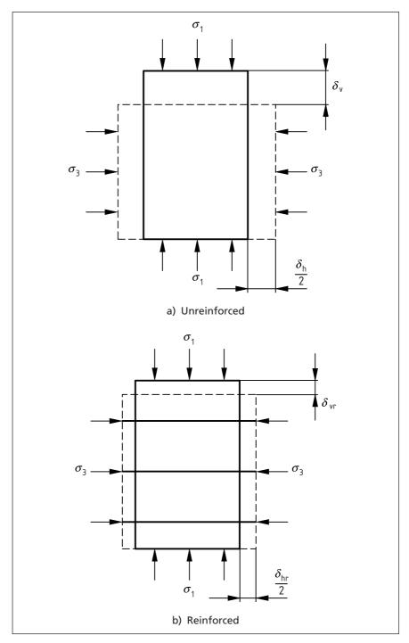
In the above illustration, both reinforced and unreinforced samples are subjected to the same magnitudes of externally applied load and the addition of reinforcement decreases deformations compared to the unreinforced soil. The addition of reinforcement will also improve soil strength.
