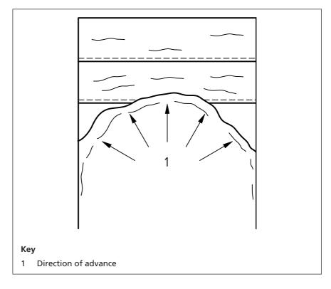
Figure 89 Construction of a "U" shaped leading edge
