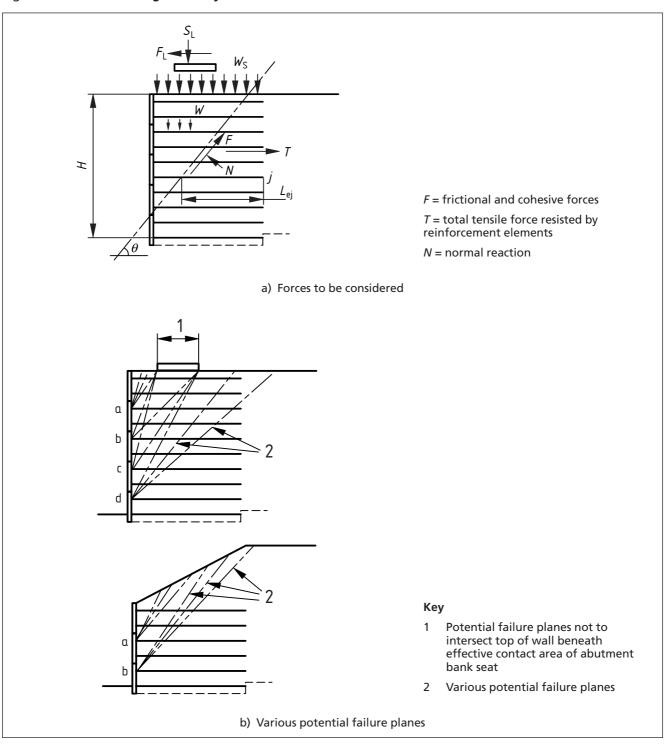
Figure 34 Internal wedge stability analysis of simple problem
