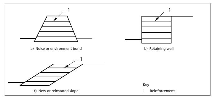
Figure 11 Examples of structures in category 2 – Applicable to walls and slopes
