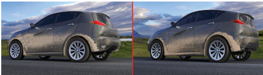
Dirt deposition on side and rear of a vehicle (left) and after aerodynamics' modification (right), with side body coverage noticeably decreased and rear area soiling slightly increased. This demonstrates the potential for subtle control of vehicle body soiling.
