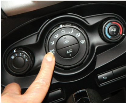
The recirculation position on the HVAC switch can shut off outside air. With the “Max A/C” label, it’s the hot-weather choice.
