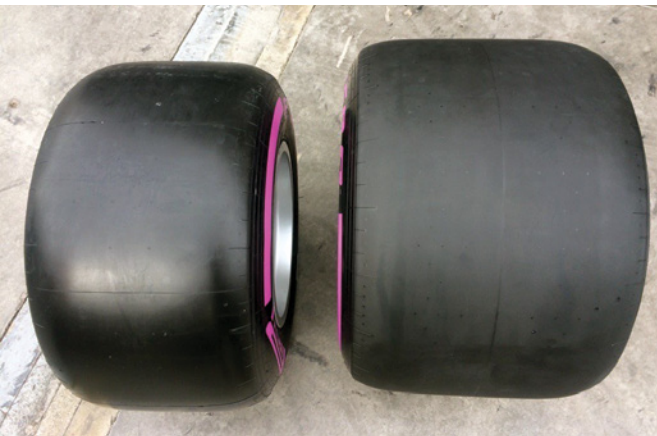
The 305 mm front and 405 mm-wide 2017-spec rear tire give this season's driver huge contact patches (image: Pirelli).
