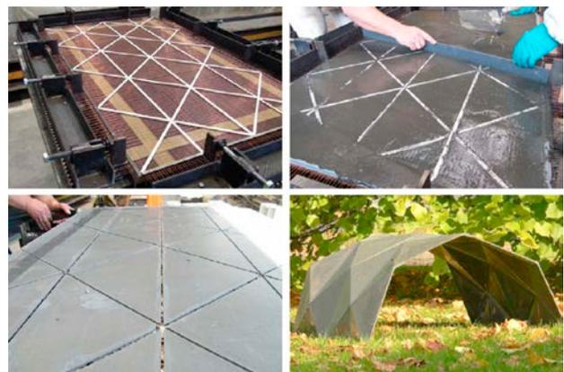
Figure 18: Manufacturing of a TRC oricrete structure [photos: Jan Dirk van der Woerd, RWTH Aachen], [45]
