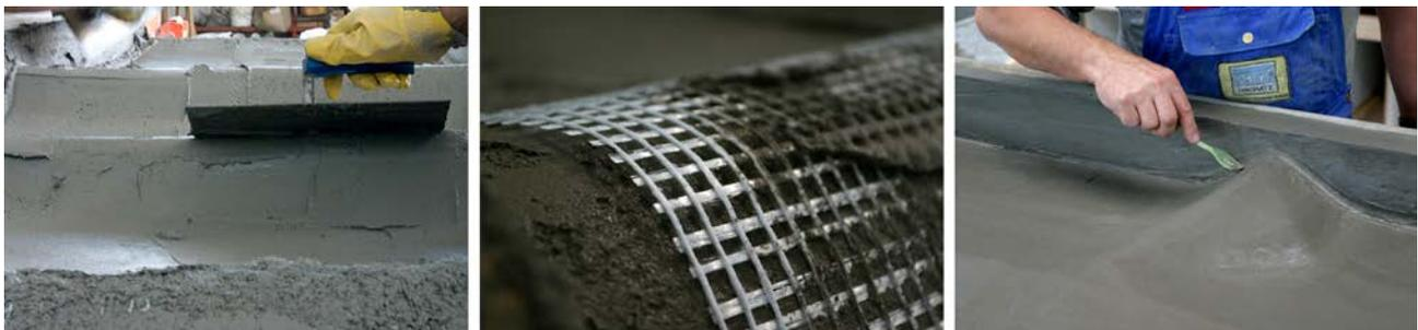
**Figure 5:** Manufacturing of a bridge segment: modeling a fine grained concrete layer, placing of the textile; final smoothing of the surface [photos: Dirk Jesse & Harald Michler, TU Dresden], [28]
