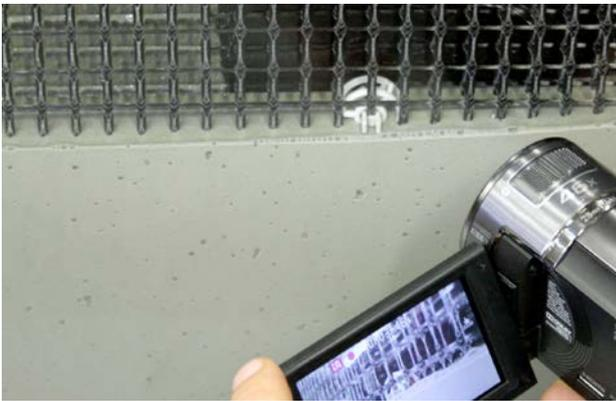
**Figure 2:** Production of TRC in casting method, here during an experiment in the laboratory, where a plexiglass formwork was used [photo: Tobias Walther, TU Dresden]
