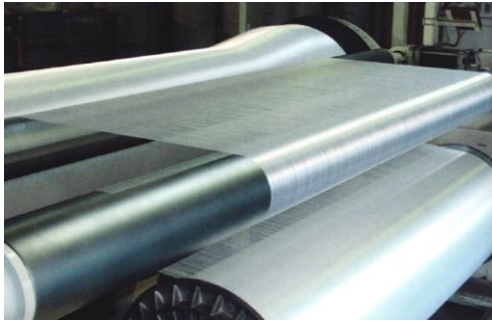
Production of a fiberglass fabric Pudenz (2004)
